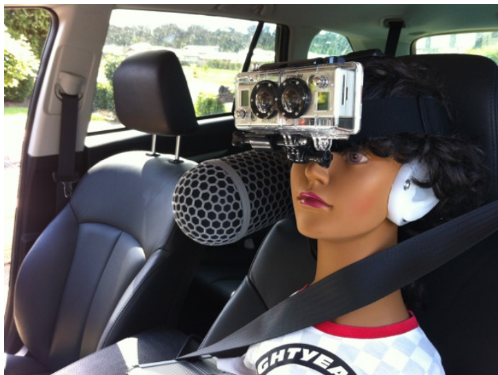
Figure 4: Binaural head with 3-D GoPro camera attached and Soundfield microphone
