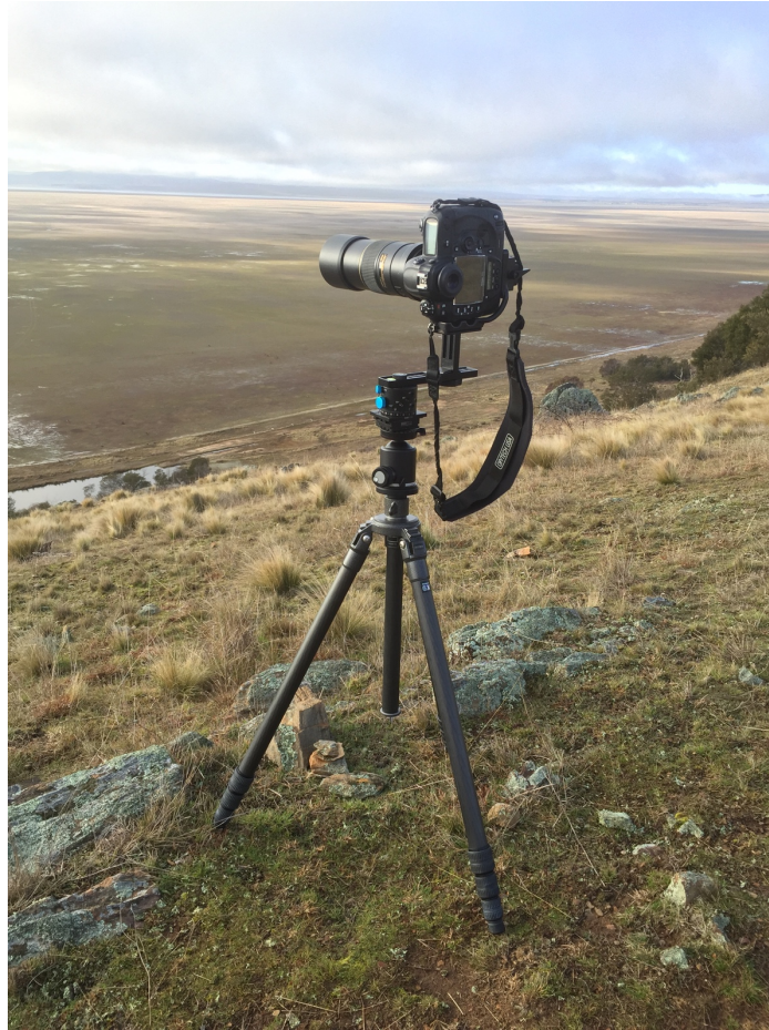
Figure 15. On site with Nodal Ninja 360° Panoramic photographic tripod head and Nikon D3x with 300mm telephoto lens. 2015
