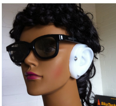
Figure 5: Custom made binaural head using mannequin head, silicon ears and condenser microphones inside ear canals.
