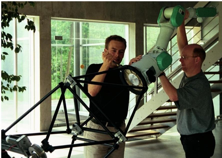
**Figure 1.** 10 degrees of freedom hybrid robot.
